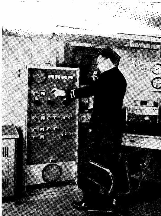
Part of the radio-room of the new Shell tanker "Drupa," showing the main Tx, a Redifon G.341, being set up by the radio officer on one of the many channels and several modes this transmitter provides. To the immediate right of the R/O, on the operating table, can be seen the matching Redifon R.408 receiver.
